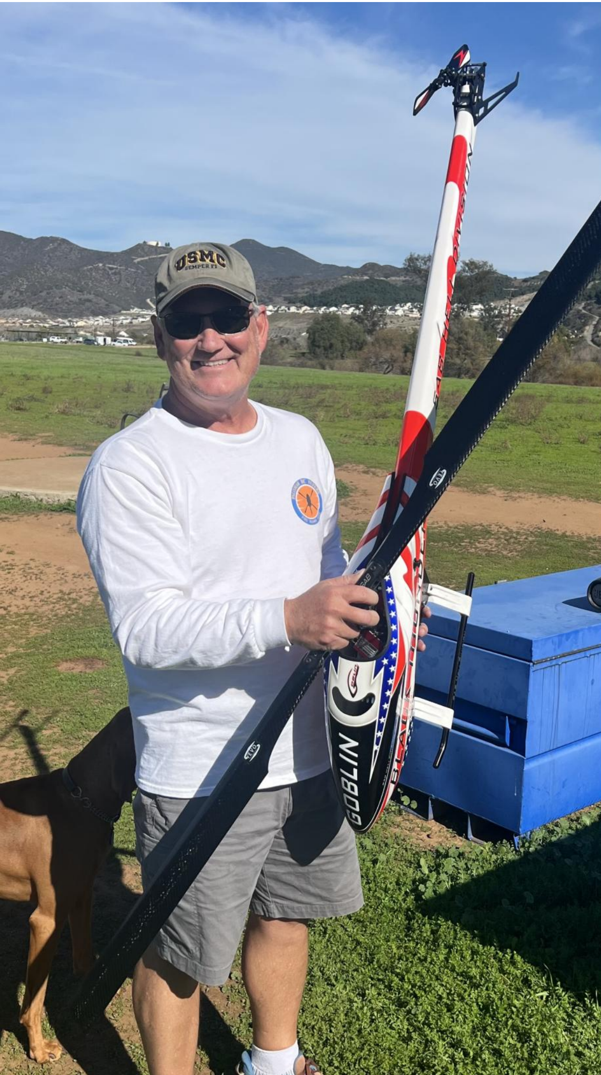
Eric Armstrong with his new OMP M7 700 size helicopter. Powered by a 200 Amp Scorpion ESC and XNova motor.
